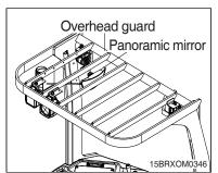
Reinforced structure of head guard is provided to guarantee the safety of the driver.
