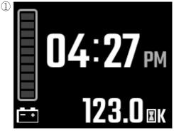
The above screen is shown when the engine is started on the truck. ESC button is pressed for more than 1 sec.
