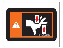
This label is attached to the mast, and provides warning on the risk of safety accidents when operating the rail, chain, sheave, fork carriage and mast.
