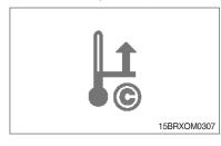
Lights up when the controller is in high temperature.
