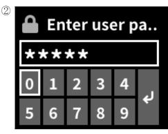
When the password input screen is shown, use the left/right button and ENTER button to enter the password.
